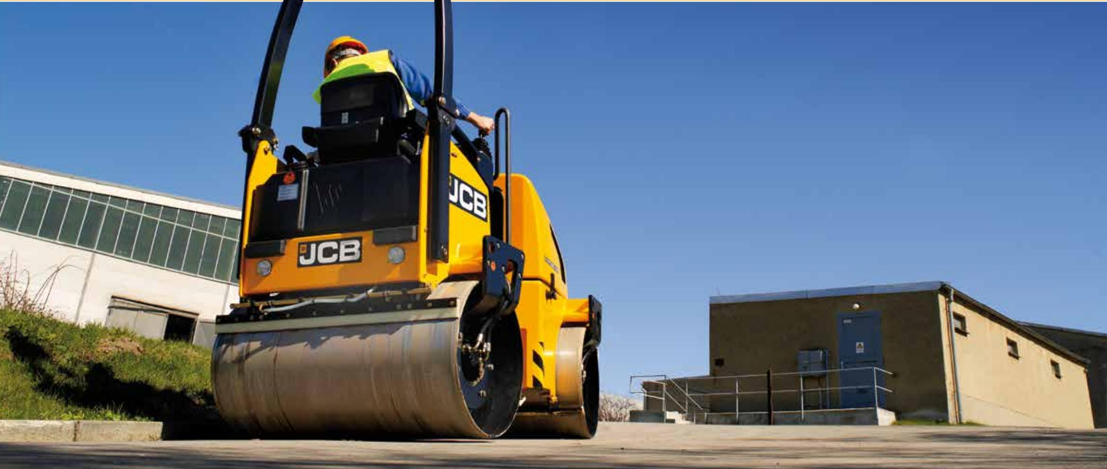
three different drum versions: 800mm, 900mm and 1000mm. The VMT260 range consists of two models: the VMT260-100 and VMT260-120, with drum widths of 1000mm and 1200mm respectively. All of these models benefit from the inclusion of a class-leading 45/95-litre diesel tank combined with a 125/230-litre water tank. This allows the VMT160/260 to work at maximum capacity for much longer than its nearest rivals, giving you over a whole working day of extra usage.
